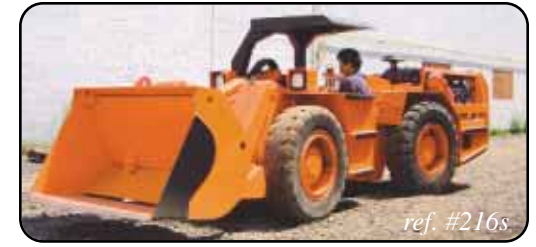
JCI 125, Deutz F4L912W, powershift transmission, ROPS canopy, fire suppression, ejector bucket, hydraulic disc brakes.... For more information call Mark Allen at Driftech Inc. 705-566-4384, fax: 705-560-8277, e-mail: mallen@driftech.com
